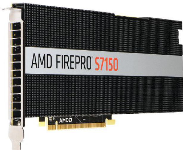
The AMD FirePro S-series takes a hardware approach to GPU virtualization, making it more difficult for hackers to break in, AMD officials say. Image courtesy of AMD.
